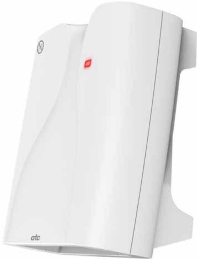
The ATC Bavaro bathroom downflow heater is sleek and modern in design. The Bavaro is controlled with a pullcord switch which can be used to change the output from 1000w to 2000w or off. The heater is fitted with a neon indicator, electronic thermostat, dual safety cutout and is rated IP22.
