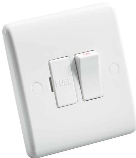
Switched fused spur units or connection units are an electrical switch with a built in fuse, designed for appliances that do not have or require a fused plug top. Fused spur units are also used for high powered electrical equipment with heavy continuous load, so that the appliance can be isolated by a single cable from a ring main for safety and maintenance purposes. 13A rated available with and without a double pole switch/neon.
